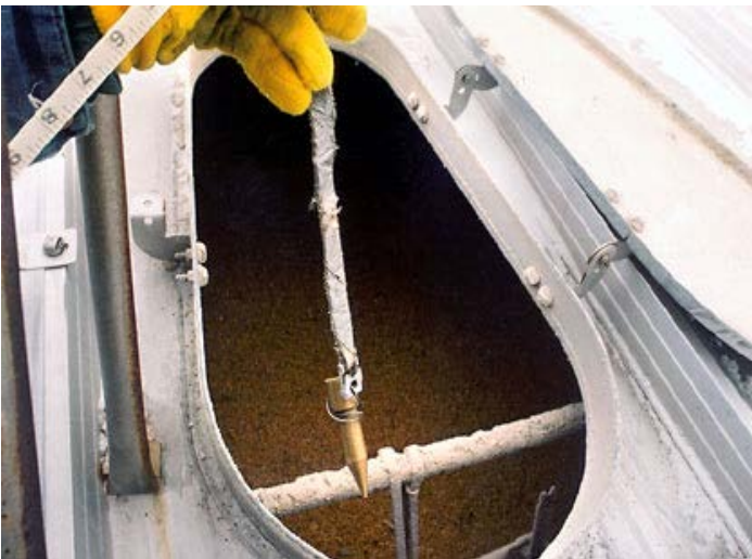
A measuring tape is used to measure airspace in a grain bin. This airspace measurement is used to determine the amount of grain in the bin.
