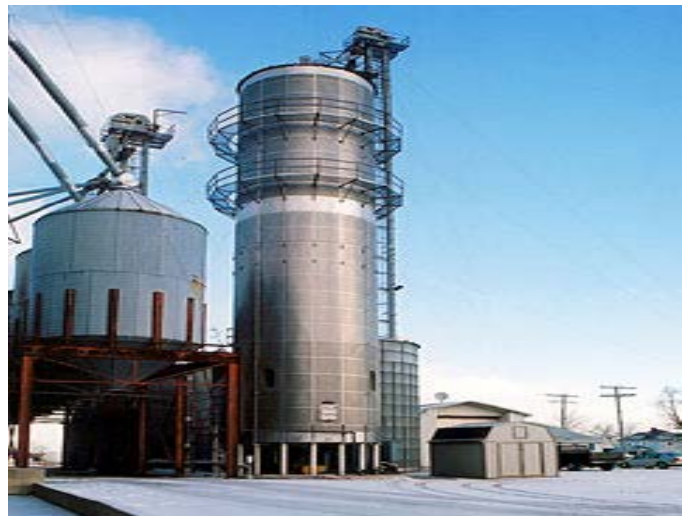
Grain dryers are used to reduce moisture content in grain and prevent spoilage during storage.
